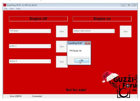
To reset the Autolearning parameters (ECU fuel trims), using the drop-down selection box, select 'Reset autolearning parameters', then click 'Start'.
