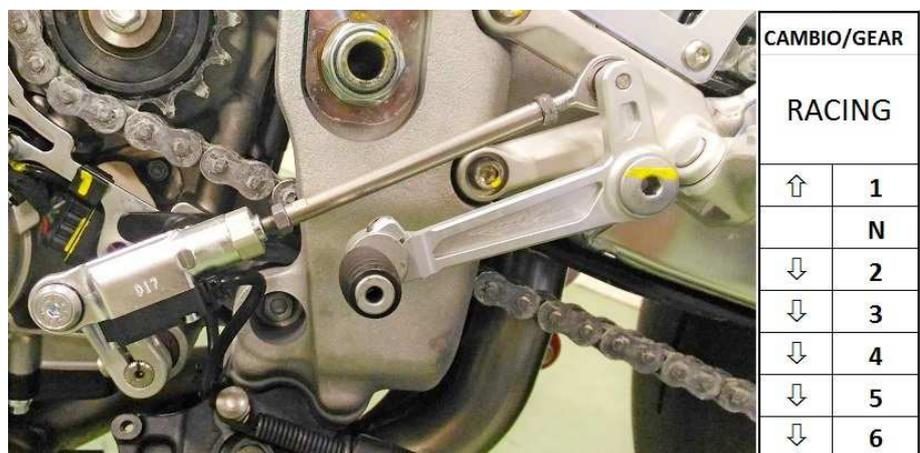
As you can see from the photo above, with the new gear lever mounted on the footpegs, the gear shaft connecting to the sensor is now raised compared to the fulcrum of the pilot footpeg, this way the transmission is reversed (racing), with the sensor still mounted in the correct position.
